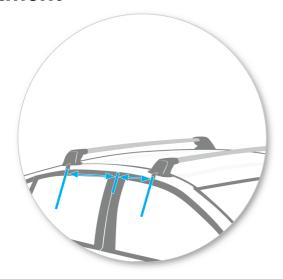
Place crossbar on vehicle. Minimum recommended spacing between the bars is 700mm (unless otherwise stated).
